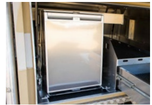
BOLT IN 110L DOMETIC UPRIGHT FRIDGE MOUNT
