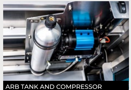
ARB TANK AND COMPRESSOR
